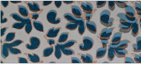
Fig. 1. An example shows that direct printing cannot achieve satisfying results. The ink-design pattern does not align perfectly with the stitch contours.
