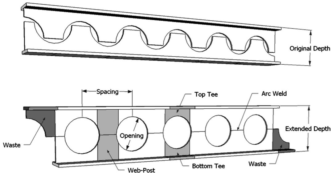
Fig. 1. Typical profiling of cellular beams.
