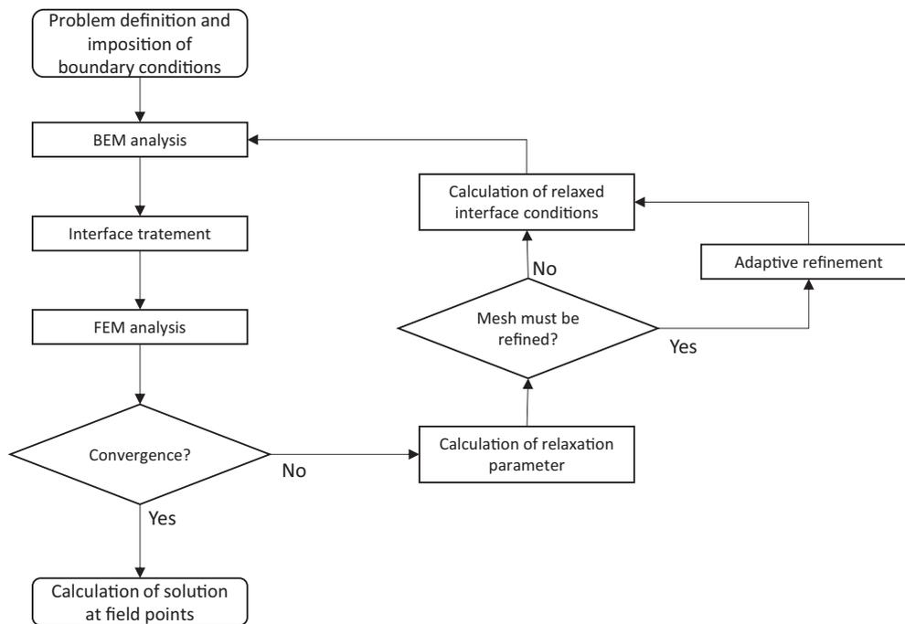
Fig. 1. Workflow of the proposed adaptive-iterative coupling approach.
