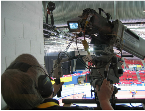
Fig. 1. Camera with sensors on lens and pan/tilt mount for virtual graphics overlay.
