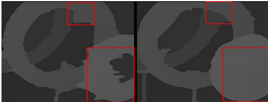
Fig. 2. Depth maps contain inconsistent errors across views. The depth values in the red windows are not consistent in both views. (For interpretation of the references to color in this figure legend, the reader is referred to the web version of this article.)
