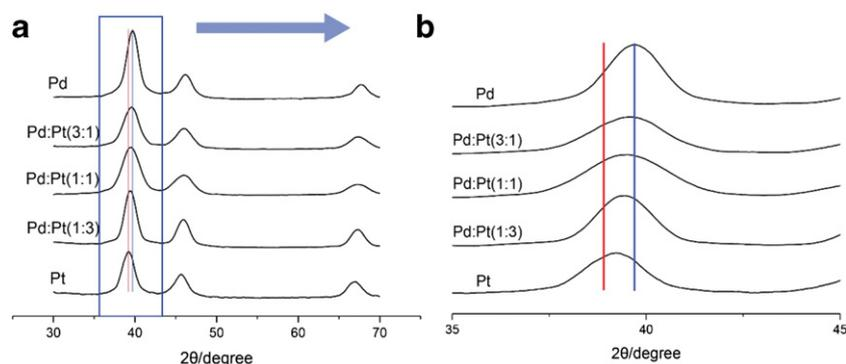
**Fig. 2.** (a) XRD patterns of the alloy seeds without the Au shell, containing Pd NPs, PdPt (Pd:Pt = 3:1) NPs, PdPt (Pd:Pt = 1:1) NPs, PdPt (Pd:Pt = 1:3) NPs and Pt NPs. (b) Parts of the XRD patterns from  $25^\circ$  to  $45^\circ$ .
