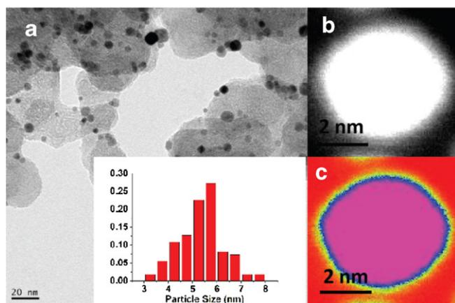
**Fig. 1.** (a) TEM image of carbon-supported PdPt@Au (Pd:Pt = 1:1) NPs. The average size of the sample is 5.36 nm. (b) HAADF-STEM image of the sample. (c) Pseudo-colored HAADF-STEM images of the sample. The purple section is the alloy core and the blue section is the Au shell.
