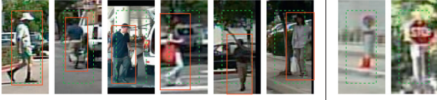
Fig. 1. Some proposal sample images which include some context around the proposed bounding boxes (dotted green rectangles). The red rectangles indicate the ground-truth bounding boxes. The sizes of the proposed bounding box and the extended box are 100 \times 41 and 128 \times 64 , respectively. The first six images include pedestrians and the last two images do not. (For interpretation of the references to color in this figure legend, the reader is referred to the web version of this article.)
