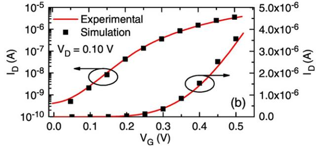
Fig. 2. MOSFET structure showing the channel doping (a). Experimental (black squares) and simulated (red lines)  $I_D$ - $V_G$  curves of the device (b). The nominal  $V_{th}$  of the device was 0.37 V and the estimated EOT was 1.5 nm. (For interpretation of the references to colour in this figure legend, the reader is referred to the web version of this article.)
