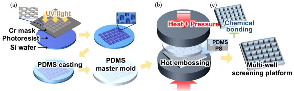
Fig. 1. The schematics of multi-well screening platform fabrication procedure. (a) PDMS mold fabrication. (b) Replication of micrometer-scale topographies into the PS bottom plate with PDMS mold. (c) Chemical bonding of the PS bottom plate with a PMMA partition.
