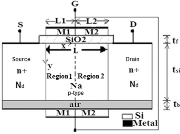
Fig. 1. 2-D Cross-sectional view of the Proposed DMDG SON MOSFET.
