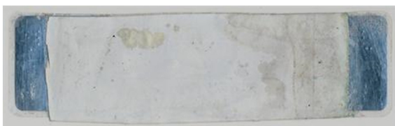
Fig. 2. A sample with bare side parts prepared for resistance measurement.
