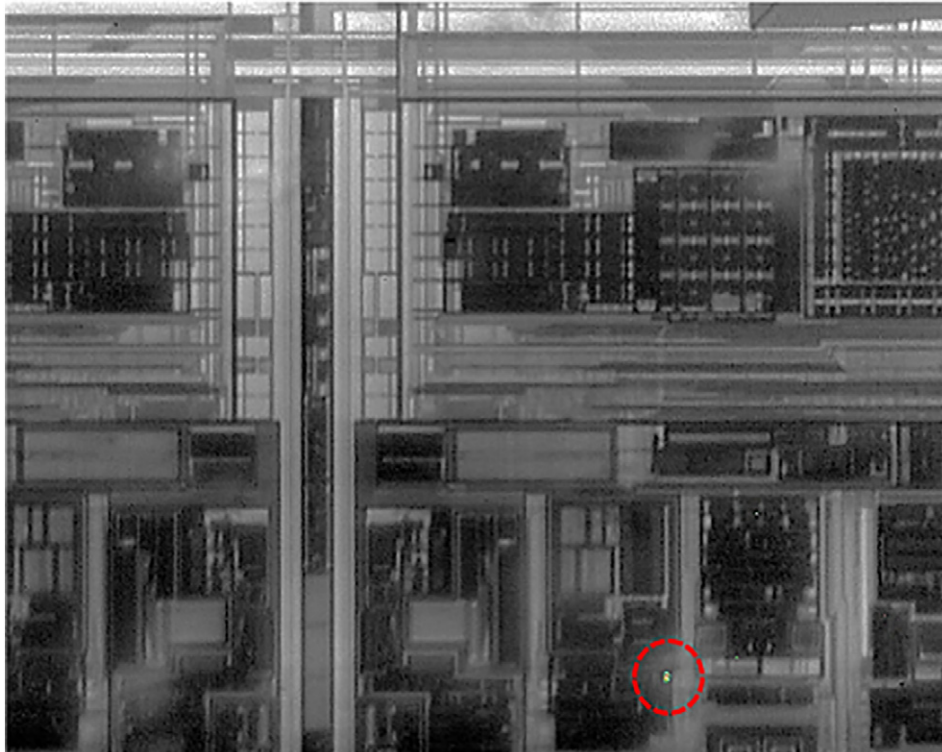
Fig. 1. The EMMI signal (circled by red line) is localized by applying the electrical condition to bias the failed device in the specific operational mode.
