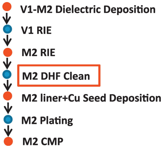
Fig. 3. Via 1 – metal 2 dual damascene process flow.
