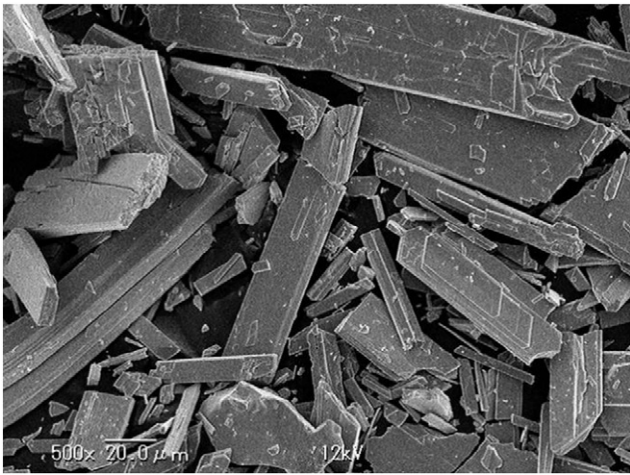
Fig. 1. SEM images of the fabricated h-WO 3 powder.
