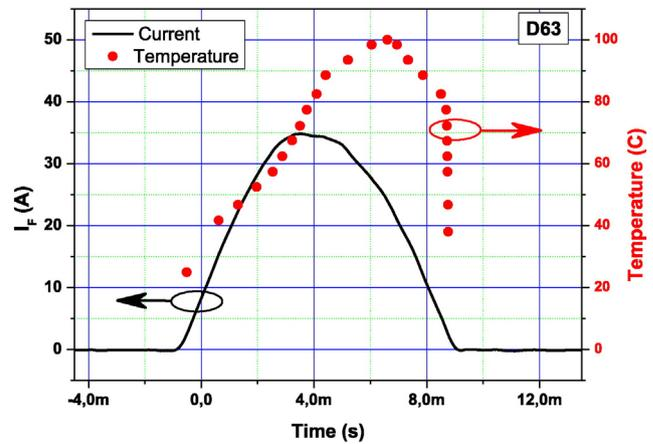
Fig. 3. Delay of the temperature versus the applied current pulse.
