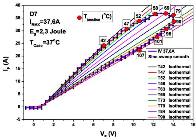
Fig. 2. Example of temperature evaluation method on the hysteresis  $I$ - $V$  curve.
