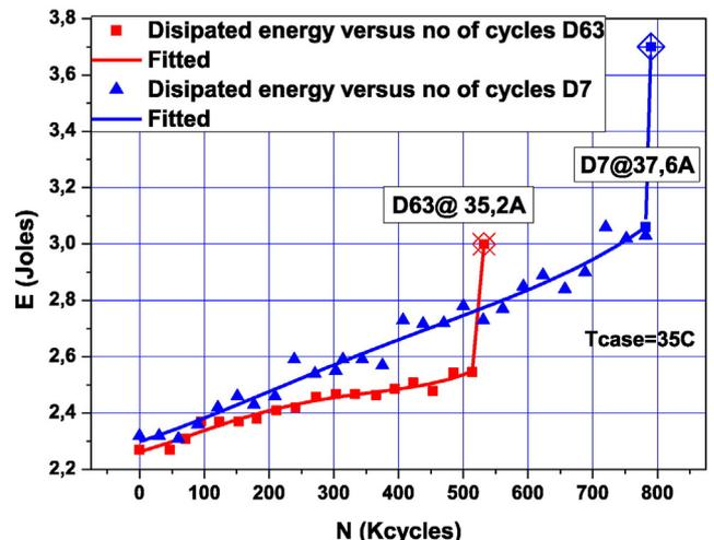
Fig. 4. Lifetime test. Evolution of dissipated energy versus the applied number of power cycling pulses.
