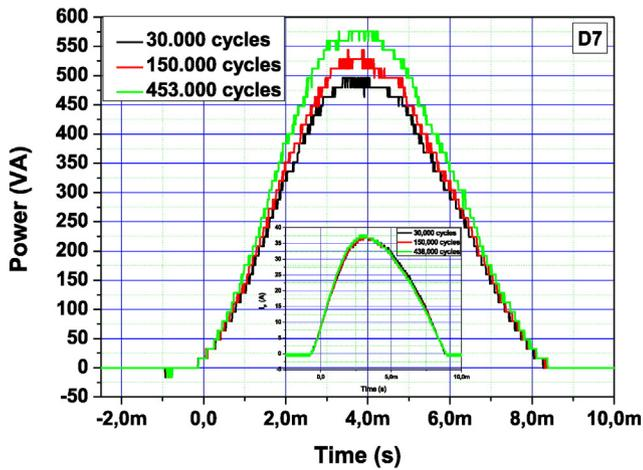
Fig. 1. Instantaneous dissipated power inside the diode after various applied test pulses.
