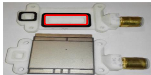
Fig. 3. The liquid cooler applied to the HBS.
