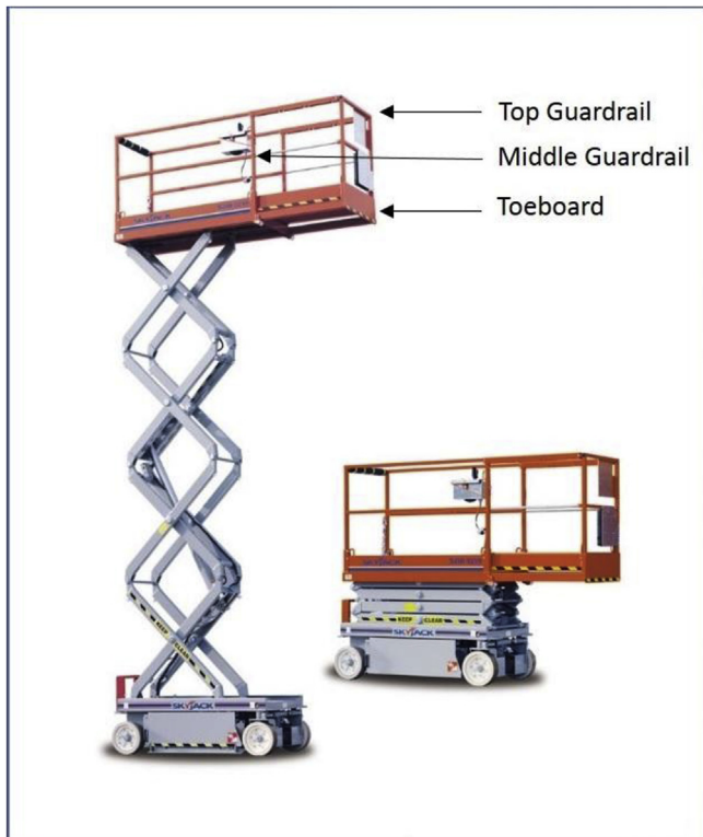
Fig. 1. A demonstration of the structure of scissor lifts (reprinted with permission of Skyjack Inc.).
