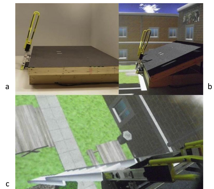
Fig. 1. Experimental setup in the Virtual Reality system. (a). Physical model of a roof and a walk-through ladder top – in the CAVE VR system; (b). Sloped roof integrated in a virtual environment; (c). View over the edge of a two-story roof at the “hybrid” real-virtual model of extension ladder.
