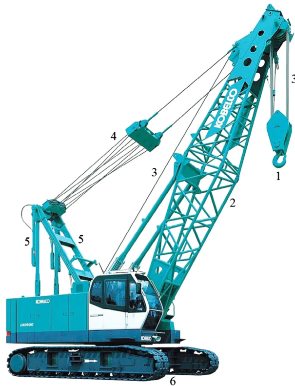
1. Hook, 2. Boom, 3 Payload-hoisting cables, 4. Boom-luffing cables, 5. A-shaped frames, 6. Crawler moving mechanism.
