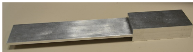
Fig. 1. Specimen of analysis: stepped cantilever bar.
