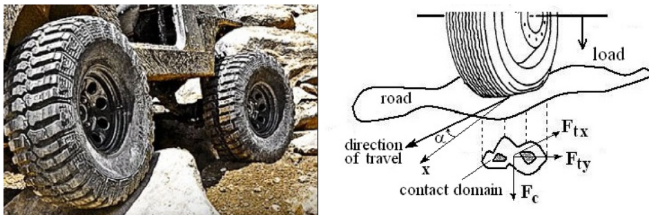
Fig. 1. Scheme of the contact tire/off-road.
