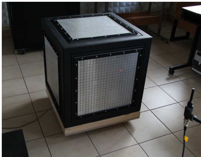
Fig. 1. Photograph of the cubic casing with a rigid frame.
