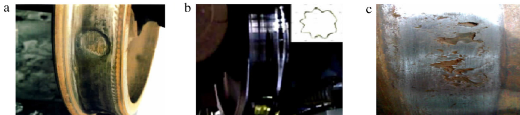
Fig. 1. Wheel shape errors: (a) flat, (b) polygonal wear and (c) tread spalling.
