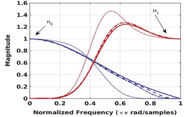
**Fig. 1.** Frequency response of filter pair [H's] for A-16/28, B-16/28, MMF-16/28 and TFOOL-15/29. Solid line: B-16/28, dashed line: A-16/28, dotted line: MMF FB, dash-dot line: TFOOL-15/29.
