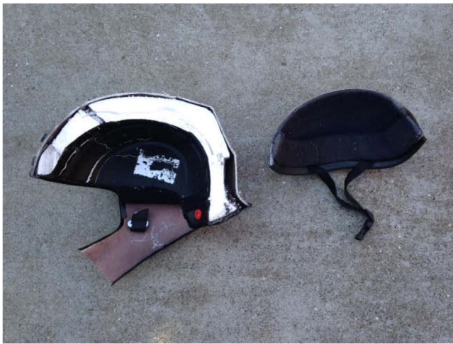
Fig. 1. Bisectional view of full-face and novelty helmet construction.
