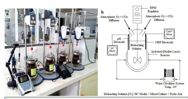
Bioreactor operating under natural diffusion of atmospheric O<sub>2</sub> & CO<sub>2</sub>
