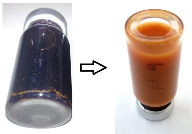
Fig. 1. O_2 generation during FeO_4^{2-} decomposition with vial explosion to release pressure at the end.
