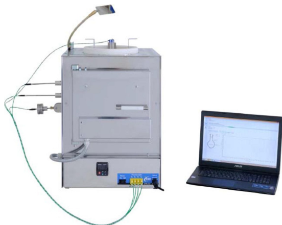
Fig. 1 – AITTA 551 auto-ignition temperature tester.
