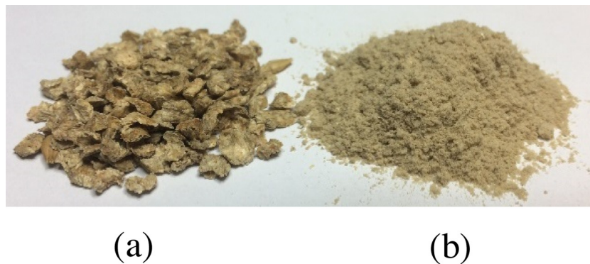
Fig. 2 – The material used in the experiment is a mixture of coarse (a) and fine (b) particles mixed with the mass ratio of 10:1.
