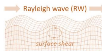
FIG. 1. A surface Rayleigh wave (RW) propagating as an acoustic wave on the surface of a deformable solid. Surface RWs supported by shear rigidity do not penetrate deeply the bulk, decaying over distances comparatively shorter than bulky shear waves, which spread in the three dimensions. Surface RWs propagate over long distances with a constant phase velocity (at lesser friction as compared to bulk waves). Due to the longitudinal and transverse restoring forces imposed by shear rigidity, shear-like RWs cause the surface elements to rotate in counter-clockwise motion as elliptical orbits in the planes parallel to the direction of propagation. This kinematic signature is specific of the “extraordinary” (solid-like) RWs in viscoelastic fluids, by opposite to the “ordinary” (liquid-like) waves, which make fluid surfaces to move clockwise, as capillary ripples do on the surface of liquid water. These surfing motions may be exploited to infer bulk rheology in soft solids and viscoelastic materials.
