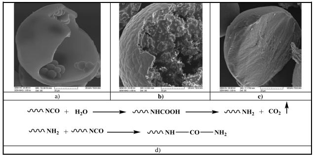
SEM micrographs of microcapsules a) before, b) after 24 h, c) after 48 h immersion in 10 wt% NaCl solution, and d) possible reactions during 48 h immersion in 10 wt% NaCl solution
