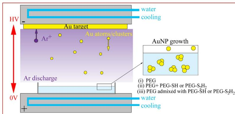
Fig. 2. Schema of preparation of PEGylated AuNPs by direct sputtering into liquid media of (i) PEG; (ii) PEG + PEG-SH or PEG + PEG-S<sub>2</sub>H<sub>2</sub> (see experimental).
