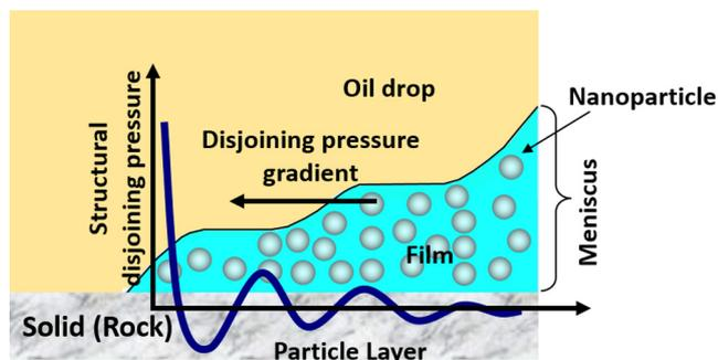
**Fig. 1.** Schematic presentation of mechanism of oil drop displacement driven by nanofluid structural disjoining pressure: Ordered layering of nanoparticles leads to disjoining pressure gradient and drives oil displacement.
