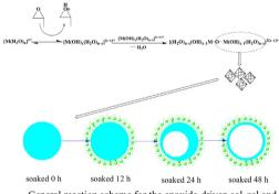
General reaction scheme for the epoxide-driven sol-gel and chemically induced self-transformation process
