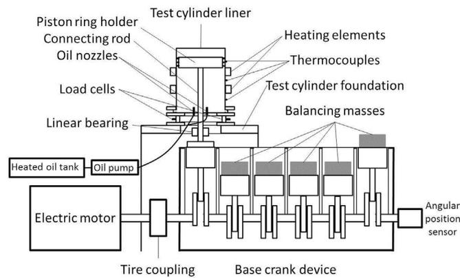
Fig. 1. Schematic view of test rig.
