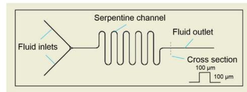
Fig. 1. Designed feature of a mold insert for fabricating microfluidic chips. (The size of the mold insert is 75 mm×25 mm. The microstructure size is 100 μm×100 μm.).
