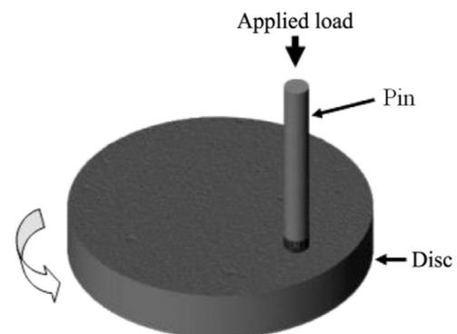
Fig. 1. Configuration of the pin-on-disc equipment [9].
