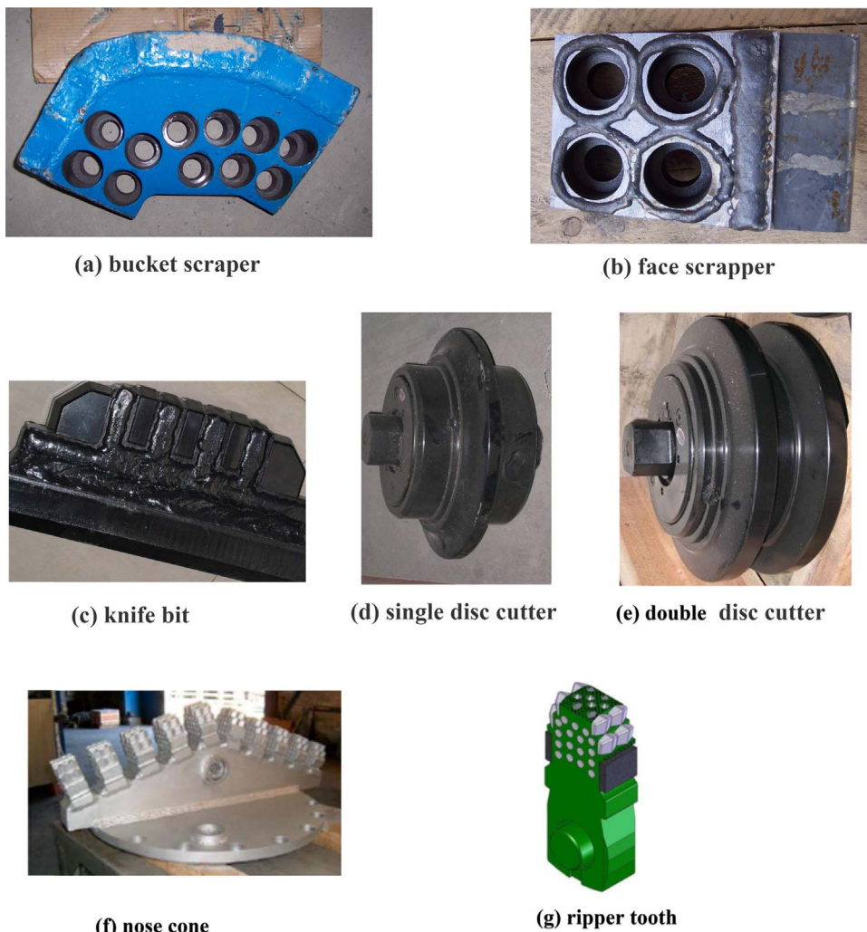
Fig. 1. Cutting tools used in soils.
