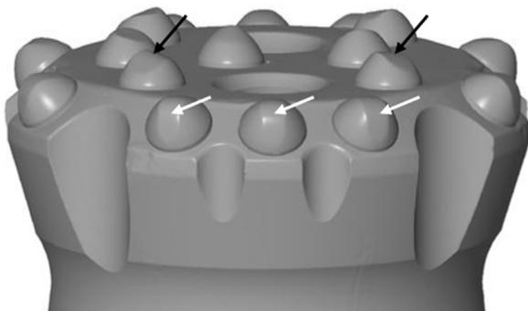
**Fig. 1.** Schematic showing the drill bit and the drill bit buttons. In the present study, two front buttons (black arrows) and three peripheral buttons (white arrows) were characterized.
