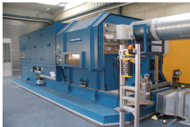
Fig. 2. Railway braking test bench - Faiveley Transport Gennevilliers.
