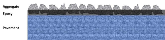
Fig. 1. Surface treatment of asphalt pavement with epoxy-bound spreading material.
