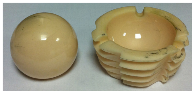
Fig. 1. A pair of retrieved in vivo alumina femoral head and acetabular cup.
