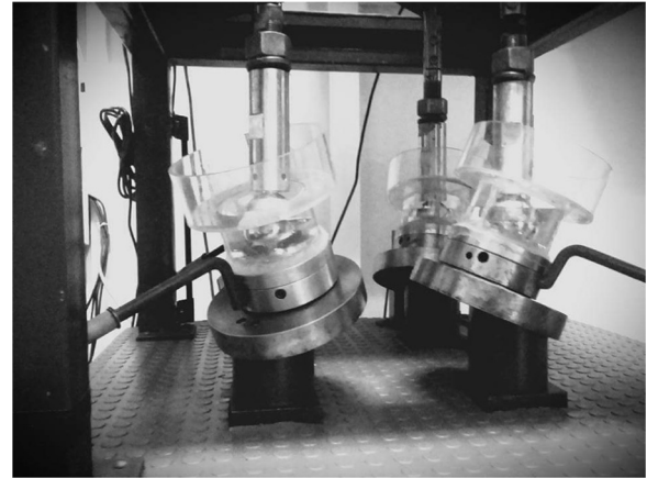
Fig. 1. Hip joint simulator FIME II [17].
