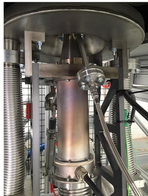
Fig. 2. Air heater used to heat the erodent carrier gas.
