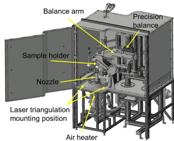
Fig. 1. CAD design of the METROSION HTSPE apparatus showing the location of the major components.
