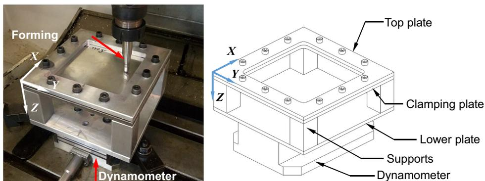
Fig. 1. SPIF experimental setup mounted on a Kyle CNC 535 3-axis milling machine.
