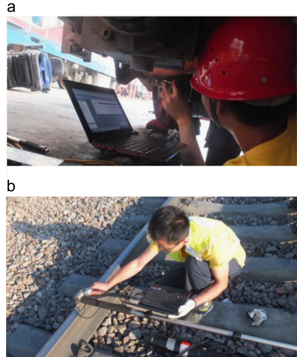
Fig. 1. Measurements of wheel/rail profile at test sites. (a) Wheel profile measurement (b) rail profile measurement.
