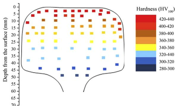
Fig. 1. Vickers hardness (HV100) data combined with the profile of the rail head.
