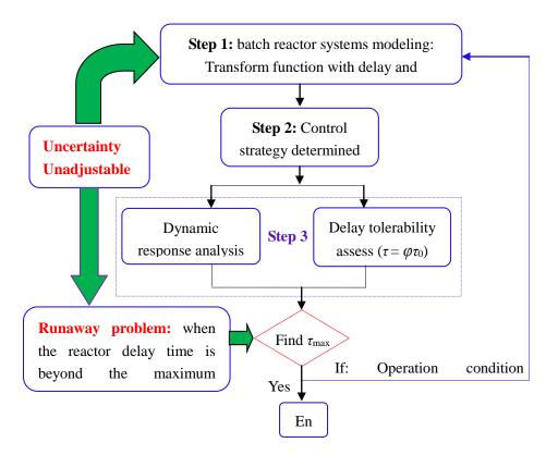
To find the maximum tolerable time delay of batch reactors, a delay tolerability index problem (DTI) is proposed based on the bisection search method combing with dynamic response analysis.
