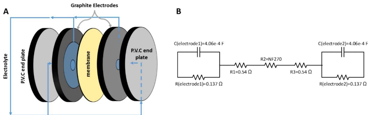
Fig. 2. Schematic structure of the electrochemical cell used for the EIS measurements (A), and the derived equivalent circuit (B). [NaCl] = 100 g/L, frequencies range – 0.1–10<sup>5</sup> Hz, effective membrane and electrodes' area – 5.76 cm<sup>2</sup>.
