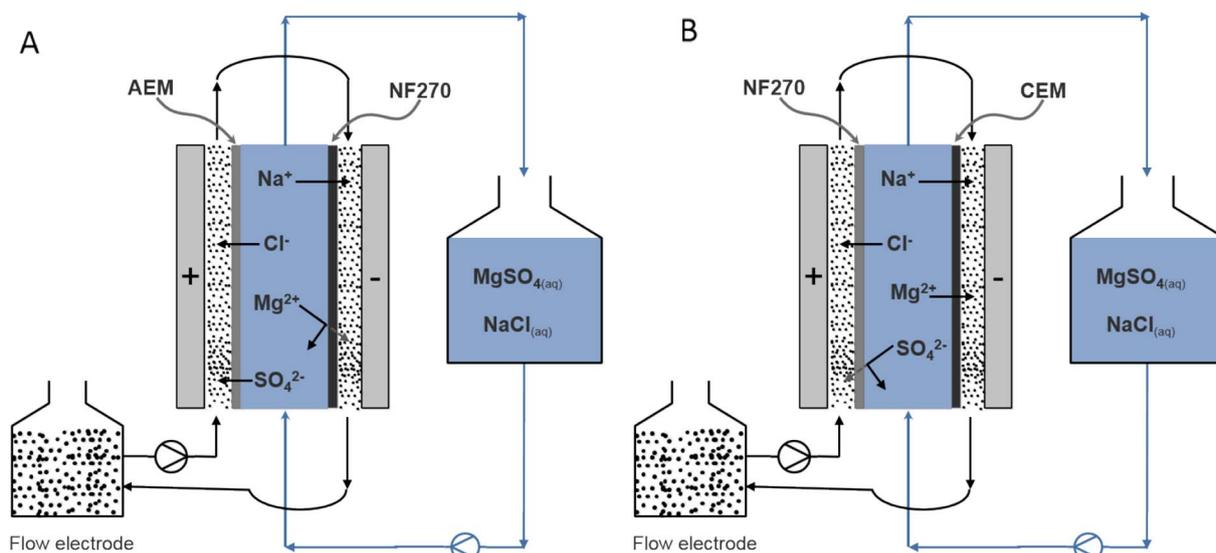
Fig. 1. Flow-electrode capacitive deionization with a nanofiltration membrane(s) and a single flow electrode for the separation of monovalent and divalent cations ((A)-AEM-NF-FCDI assembly) and anions ((B) - CEM-NF-FCDI assembly).
