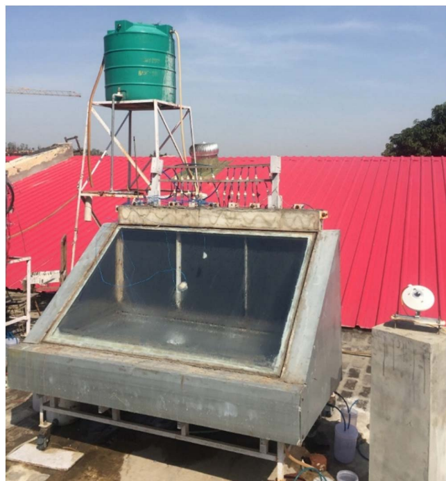
Fig. 1. Photographic view of FW-BVMED – HR solar still.
